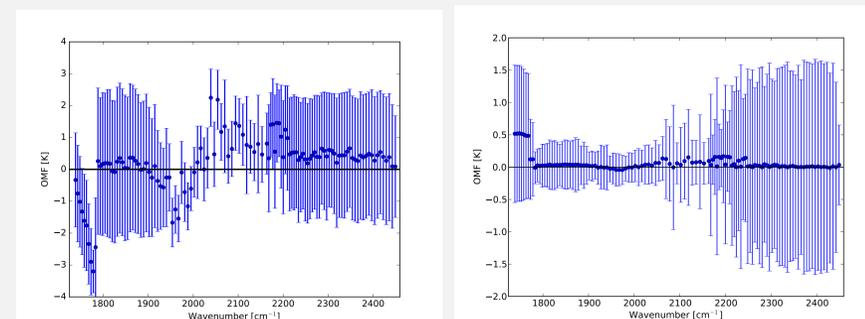
OMF and corresponding standard deviations (error-bars) as a function of MISTIC channels (left: real and right: synthetic OSSE data).
