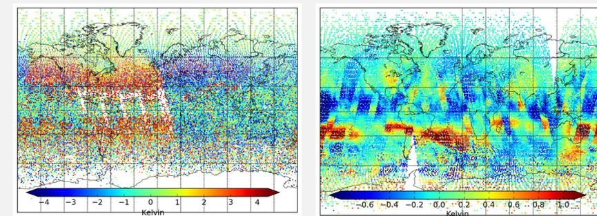
The OMF statistics for the MISTIC Chan. 2359.77  $\text{cm}^{-1}$  (left: real and right: synthetic OSSE observations). The large difference between the real and OSSE statistics is due to the NLTE.
