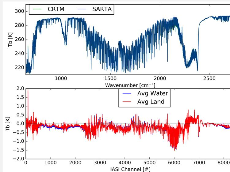
Comparison of CRTM and SARTA over land and ocean for the IASI instrument. The MISTIC instrument covers the spectrum range from 1734.70  $\text{cm}^{-1}$  to 2449.18  $\text{cm}^{-1}$  (590 channels).
