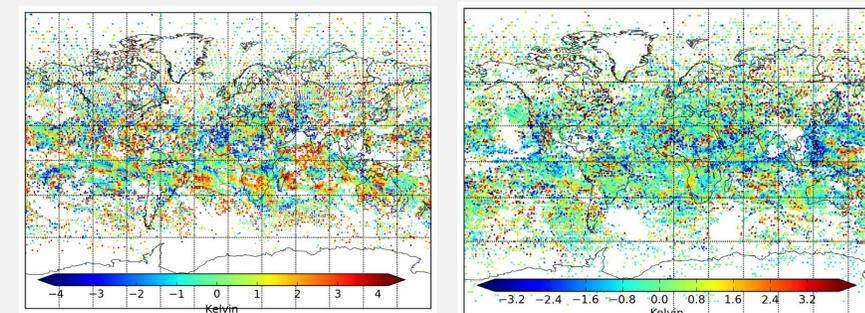
Observation minus forecast (OMF) for the MISTIC observations (Chan. 1839.15  $\text{cm}^{-1}$ ) assimilated using the GMAO GEOS-5 data assimilation system. Left panel is for the real and right for the synthetic OSSE observations.
