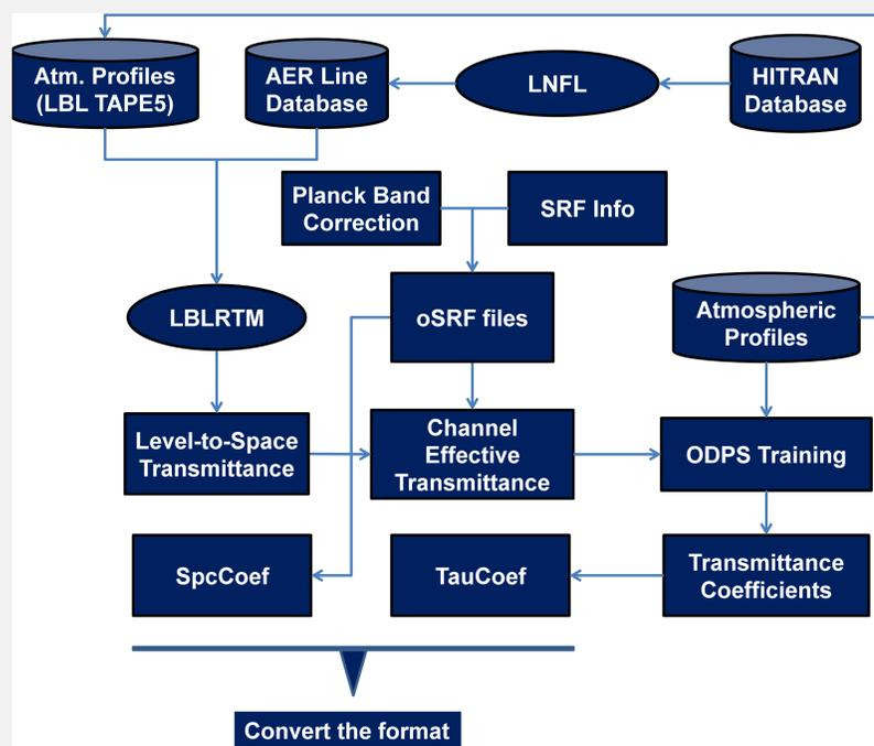
The CRTM Training process includes four major steps: (i) generating the SpcCoef files which include the sensor specific information, e.g., frequency of the channels, (ii) calculating the absorption coefficients using a line-by-line model, (iii) convolution of the absorption coefficients and the sensor response function, and (iv) regressing the sensor absorption coefficients vs. geophysical variables such as water vapor, ozone, temperature, and/or a combination of them.
