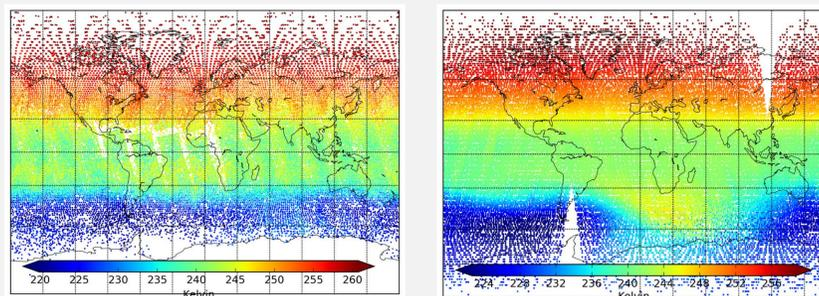
Real (left) vs. simulated (right) MISTIC observations (Channel 2359.77  $\text{cm}^{-1}$ ). Difference between the real and simulated data is due to the non local-thermal equilibrium (NLTE).
