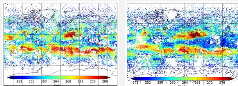
Real (left) versus simulated (right) MISTIC observations (Channel 1839.15  $\text{cm}^{-1}$ ). Synthetic observations are used in the GMAO OSSE activities. The real observations were generated from the IASI full spectrum observations.
